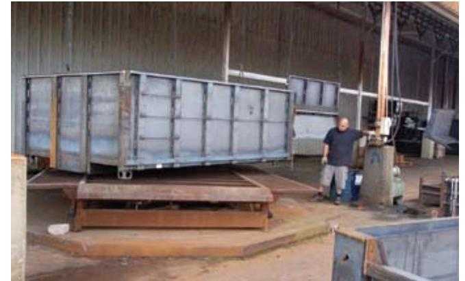
Dump bodies are transported by forklift from the assembly plant to the beginning of the conveyor line that will carry the body through the finishing process. This turning fixture accepts the dump body from the forklift and rotates it 90° so that it can more easily be attached to the conveyor line.
