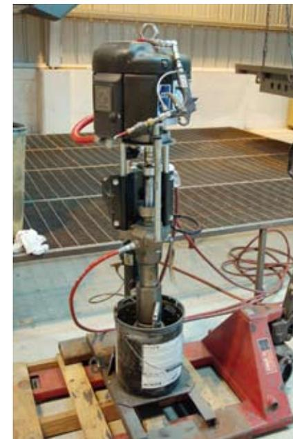
This caulk gun is used to apply heat-cured caulk to seal out water as the body comes out of the first oven. As the body cools from the oven, the caulk hardens.
