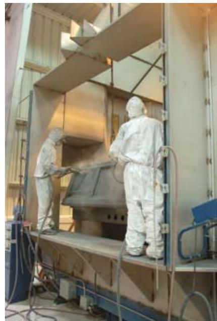
Manual application of powder supplements the 26 guns contained inside the automated spray system inside the booth.
