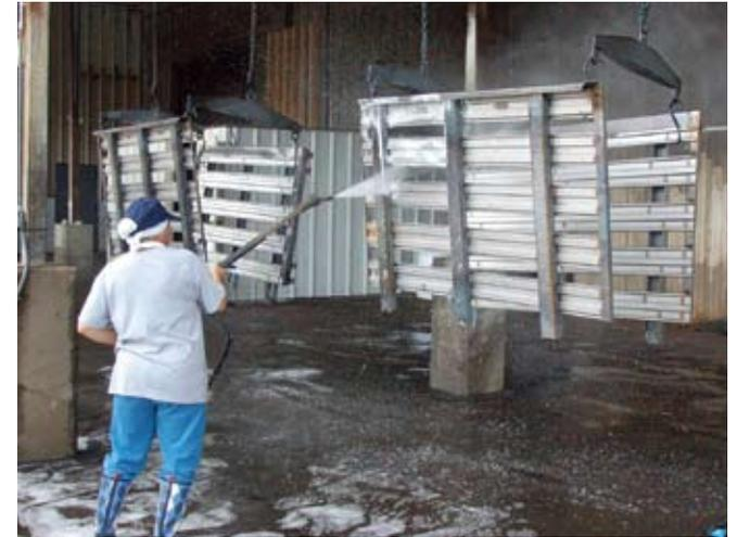
A mixture of hot water and biodegradable cleaner is sprayed to remove surface contaminants. By sending a clean body to the shot blast booth, the shot can be recycled more effectively.
