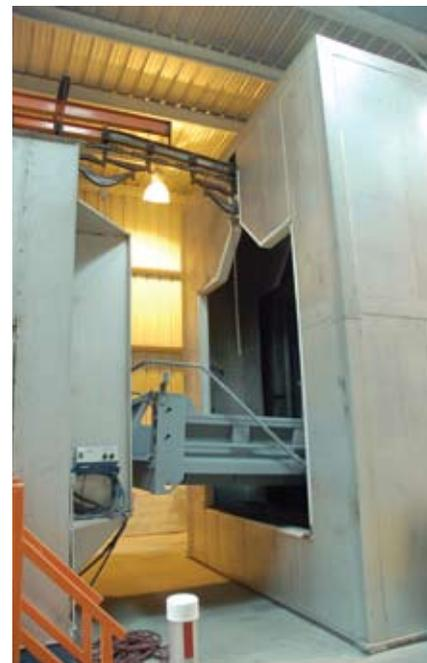
Primed bodies move into an oven that causes the powder to gel and to bond to the substrate.
