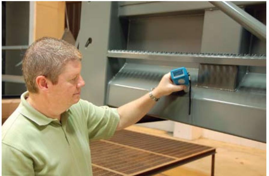
Godwin uses PPG powder coat material. During a recent visit to the Godwin plant, PPG's Mike Sloop is shown here testing the thickness of the coating. Standard specs call for the primer to be two-mils thick. Thickness of the top coat should be between three and four mils.
