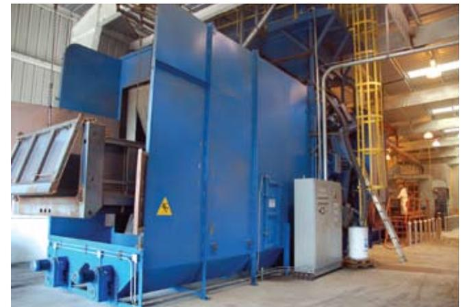
Key components of the Godwin powder coat line can be seen here. Moving at an average speed of three feet per minute, bodies move through the shot blast machine, foreground, followed by the powder coat booth and primer oven. Including the top-mounted hopper that feeds the shot, the shot blast machine is 30 feet tall.
