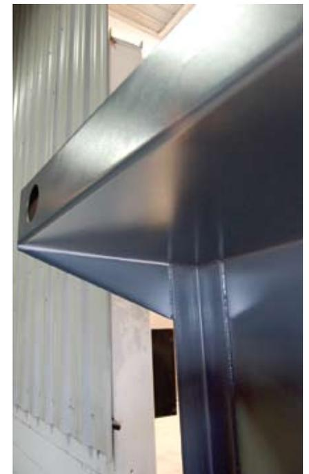
Caulked seams along the cab shield easily accept the powder top coat.
