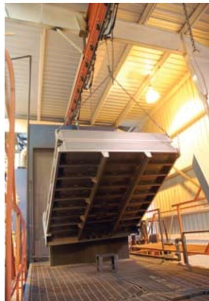
The first load a Godwin body dumps is the residual shot blast material that cleans its surface. The steel shot falls through the floor grate so that it can be collected and recycled.
