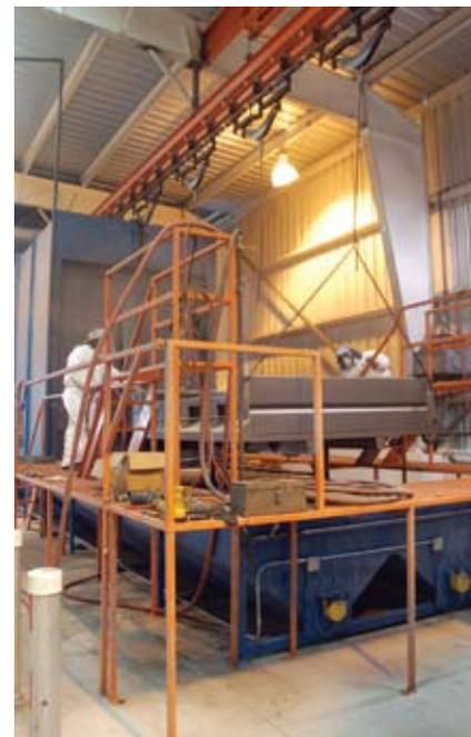
Compressed air removes the remaining shot that did not fall out when the body was hoisted up.
