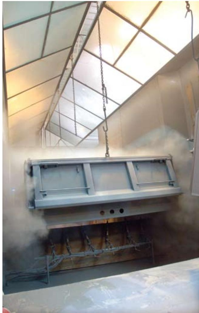
Electrostatic guns charge the powder, creating a cloud that is attracted to steel.
