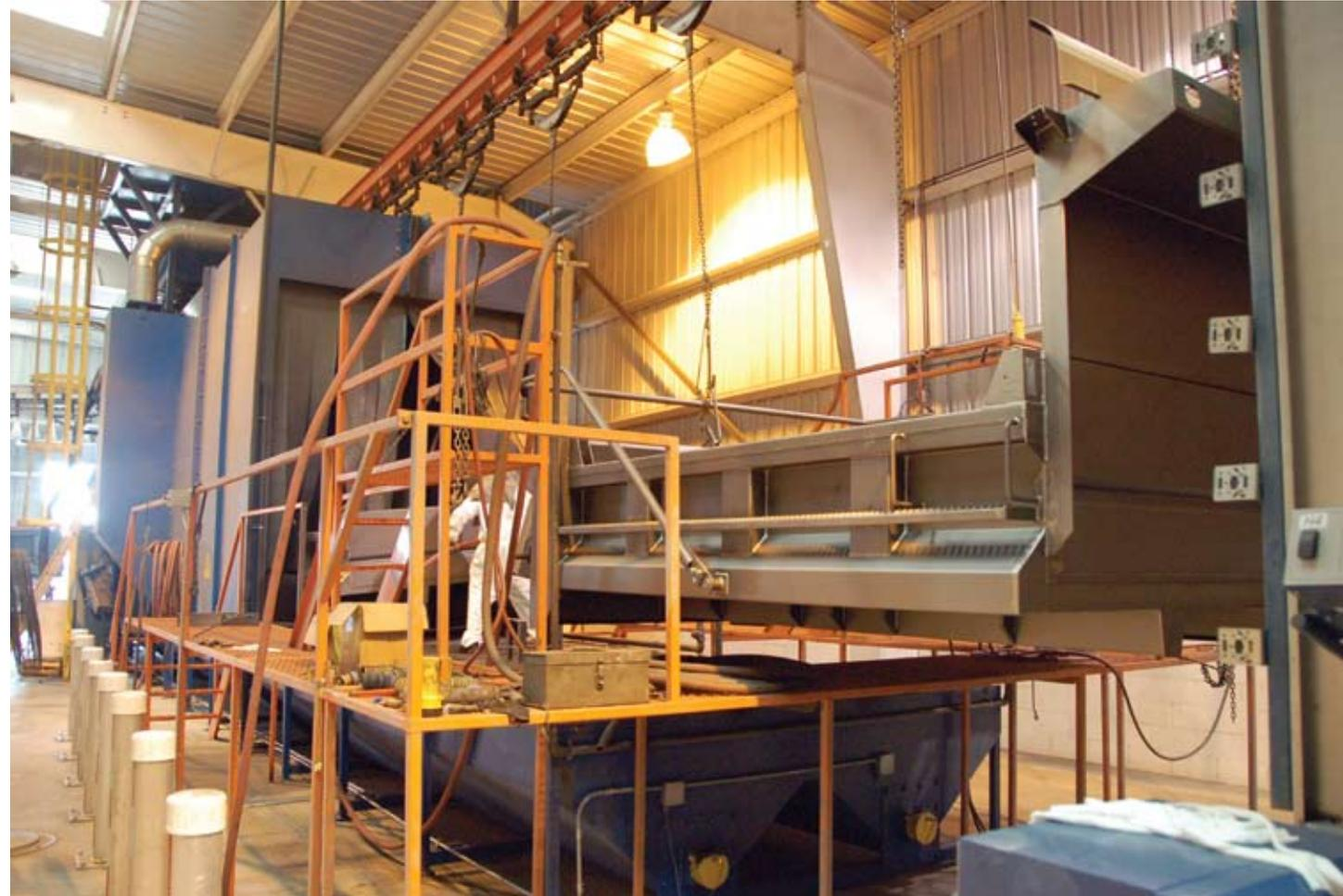
Godwin Manufacturing recently installed an automated finishing line to powder coat steel dump bodies. Shown here: a dump body leaves the new 70-ft-long Wheelabrator shot blast machine en route to the booth where a zinc-rich primer is applied.
