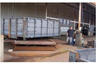
Dump bodies are transported by forklift from the assembly plant to the beginning of the conveyor line that will carry the body through the finishing process. This turning fixture accepts the dump body from the forklift and rotates it 90° so that it can more easily be attached to the conveyor line.
