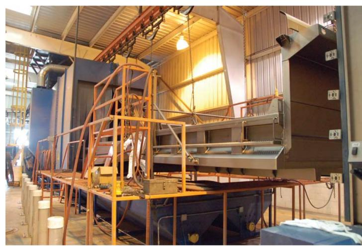
Godwin Manufacturing recently installed an automated finishing line to powder coat steel dump bodies. Shown here: a dump body leaves the new 70-ft-long Wheelabrator shot blast machine en route to the booth were a zinc-rich primer is applied.
