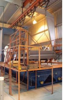
Compressed air removes the remaining shot that did not fall out when the body was hoisted up.
