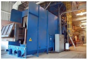
Key components of the Godwin powder coat line can be seen here. Moving at an average speed of three feet per minute, bodies move through the shot blast machine, foreground, followed by the powder coat booth and primer oven. Including the topmounted hopper that feeds the shot, the shot blast machine is 30 feet tall.
