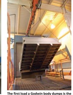
residual shot blast material that cleans its surface. The steel shot falls through the floor grate so that it can be collected and recycled.
