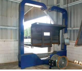
After being cleaned, forced air speeds the drying process, reducing the possibility of flash rust.
