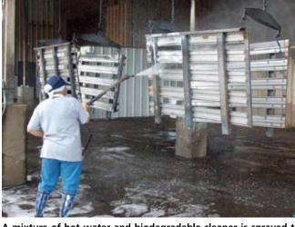
A mixture of hot water and biodegradable cleaner is sprayed to remove surface contaminants. By sending a clean body to the shot blast booth, the shot can be recycled more effectively.
