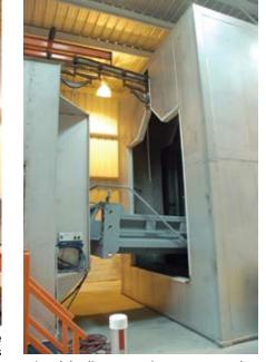
Primed bodies move into an oven that causes the powder to gel and to bond to the substrate.
